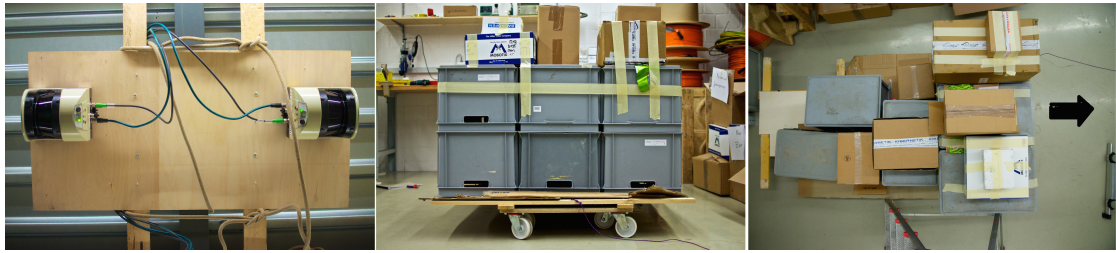
Figure 2.7: Left: The scanners were mounted to the ceiling at a height of approximately 3.4m. Center: Front of the model debris-flow platform. The string to pull the platform is visible in the lower part of the image. Right: Top-down view of the stacked boxes simulating the coarse-grained surface of a debris-flow surge head, with the greatest height at the front. The arrow indicates the direction in which the model was pulled.
