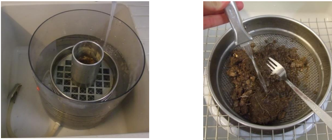
Figure 7a, b: Aggregate stability test and root cleaning. The soil sample was placed in the metal tube and then flooded. Adjacent, roots were extracted from soil which remained on the 20 mm sieve. Photos: Regula Christon.
