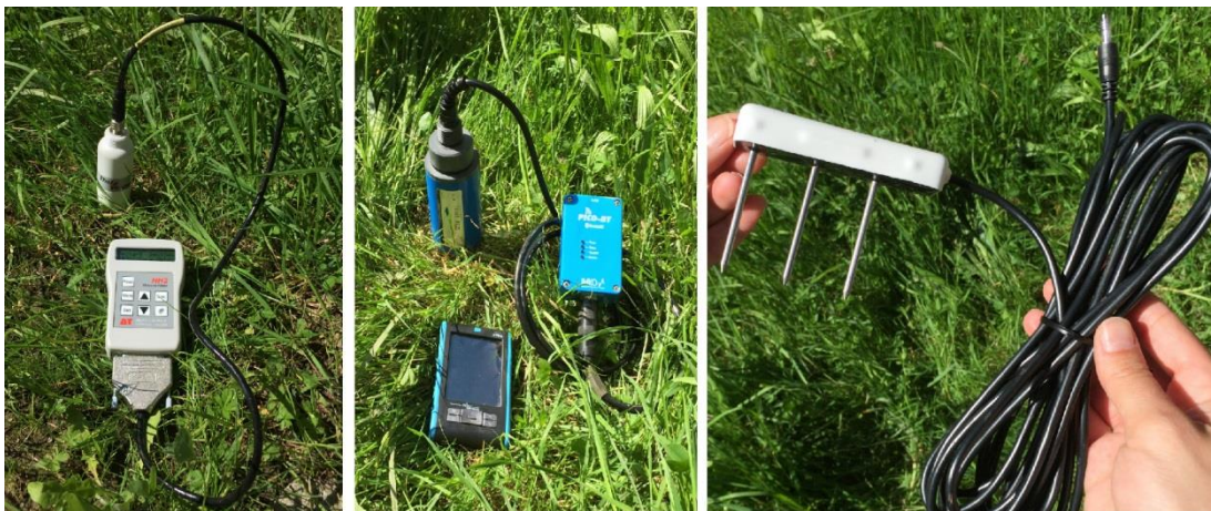
Figure 7: ML3 ThetaProbe sensor with Moisture Meter HH2 (left), TRIME-PICO 64 sensor with PICO-BT Bluetooth module and PDA (middle) and GS3 Greenhouse sensor with cable for the logger connection (right)
