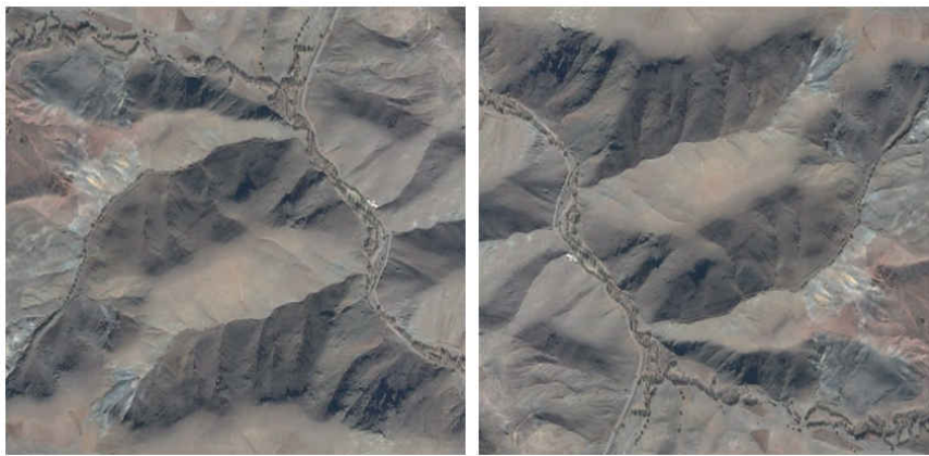
Figure 3.7: Same image. On the left side, the image is with terrain reversal effect, on the right side, the image is turned 180^\circ and the effect disappears.
