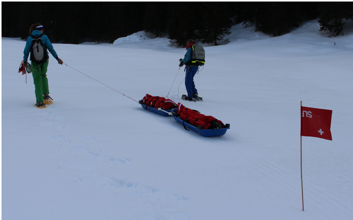
Figure 16. Measuring transect 7 at Monbiel. The GPR sledge is pulled by two people. The flag shows the location of a GPR marker, where also manual measurements were taken (photographed by Lucie Eberhard).
