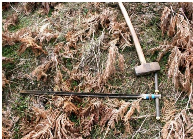
*Fig. 10 One metre long Pürkhauer used for the systematic search of ash depositis at site II and III.*
