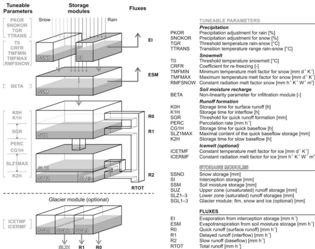
FIGURE 4.3: PREVAH model structure schematic [Viviroli et al., 2009]
