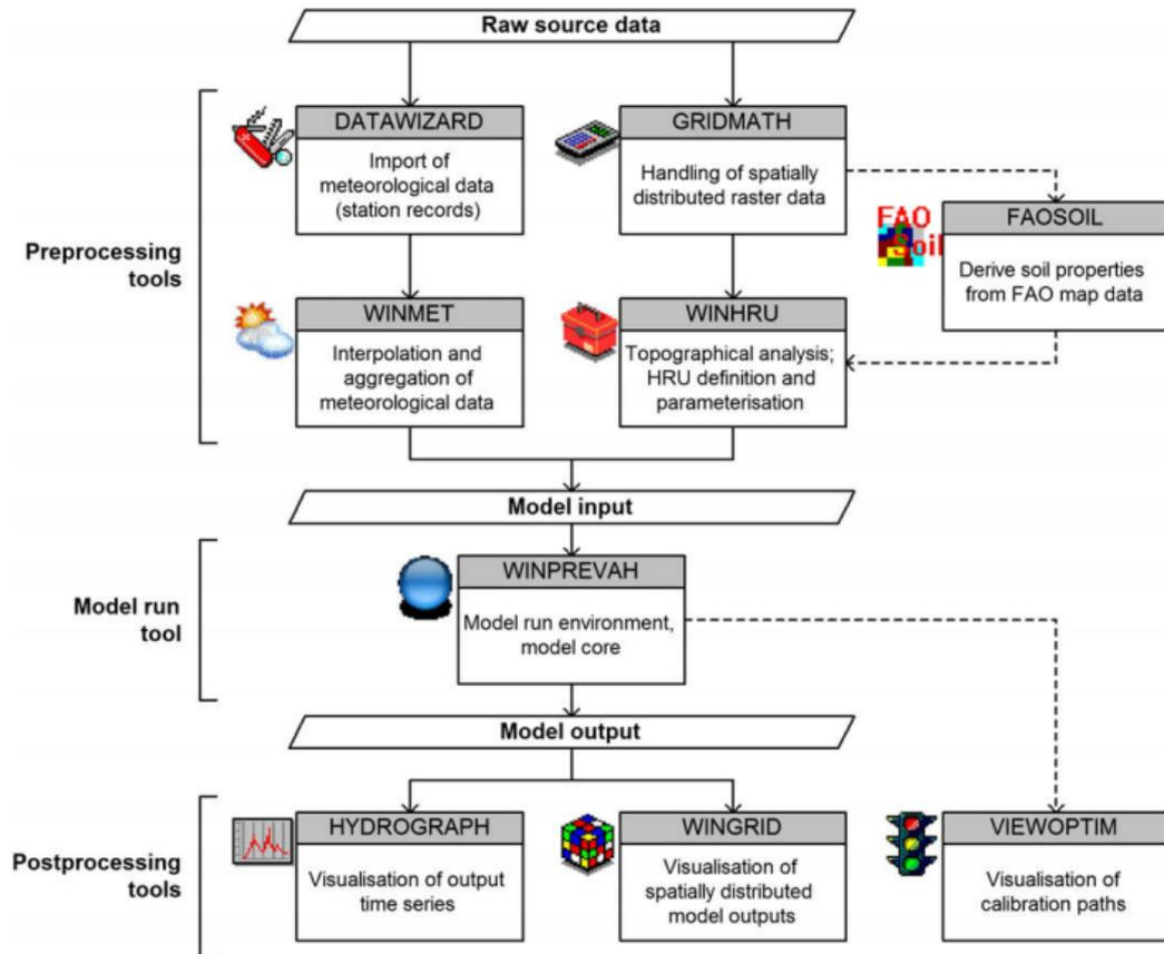
FIGURE 4.4: PREVAH's pre-processing, model run and post-processing [Viviroli et al., 2009]
