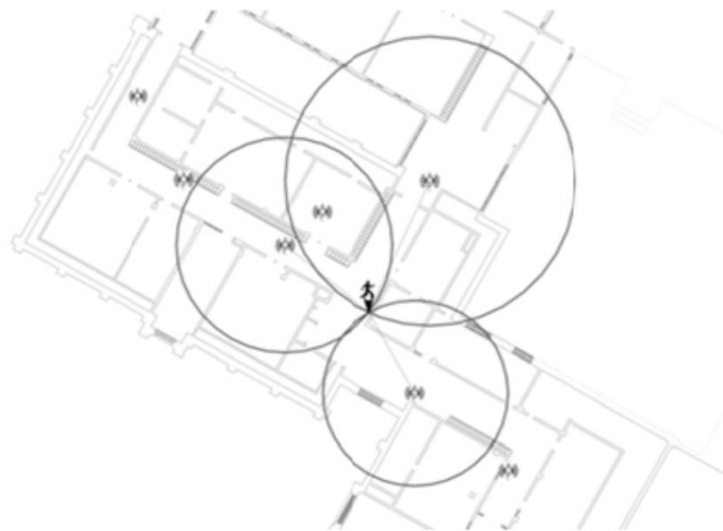
Figure 1: Distance from three APs calculated using RSSI values (Source: (Bell et al. 2010))
