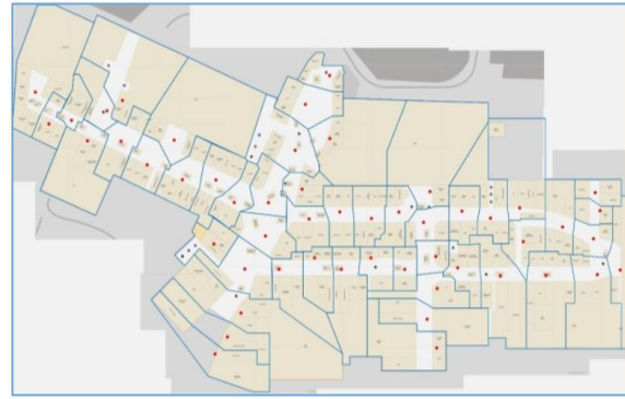
Figure 3: Adjusted Voronoi polygons respecting physical layout of the environment (Source: Bai et al. 2014)
