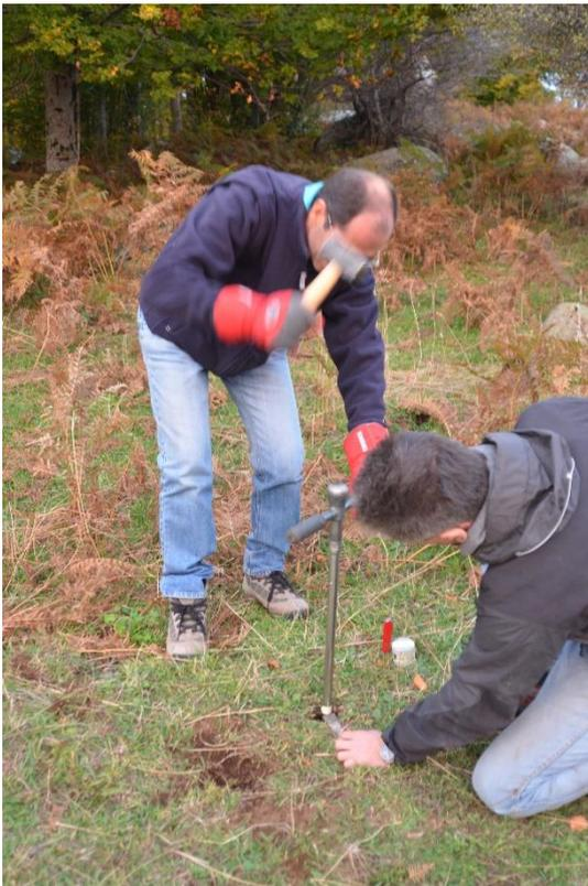
Figure 8. Soil sampling at the reference site with a core sampler. (Foto: A.Ruppli)
