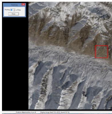
Figure 7.6: Example from the creation of moving images with StereoPhoto Maker. In the upper left corner, the flashing rate can be adapted. On the lower border the position alignment in the x- and y-
