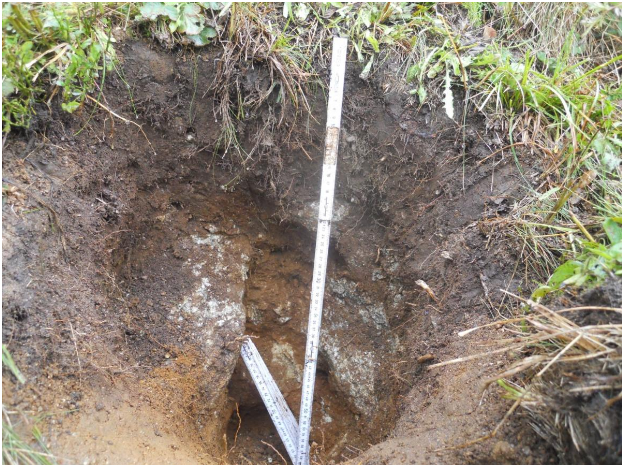
Fig. 3–1: Profile 2 with large granitic rocks (white) protruding. (A. Musso, 2015)
