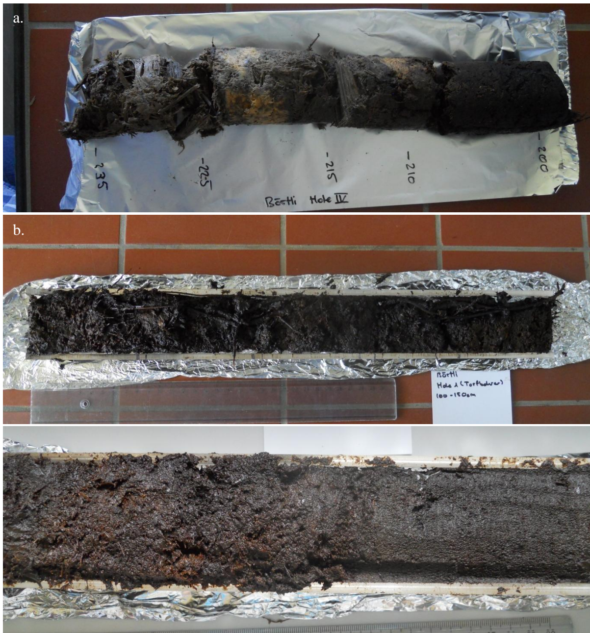
Fig. 2–3: Peat cores from Börtli A and Brätschenflue A. a. Layer of massive wood from below 200cm in Börtli A. b. Heterogeneous peat at 100–150cm with either roots or twigs in Börtli A. c. Abrupt change of peat decomposition state at 260cm in BF A. (A. Musso, 2015)
