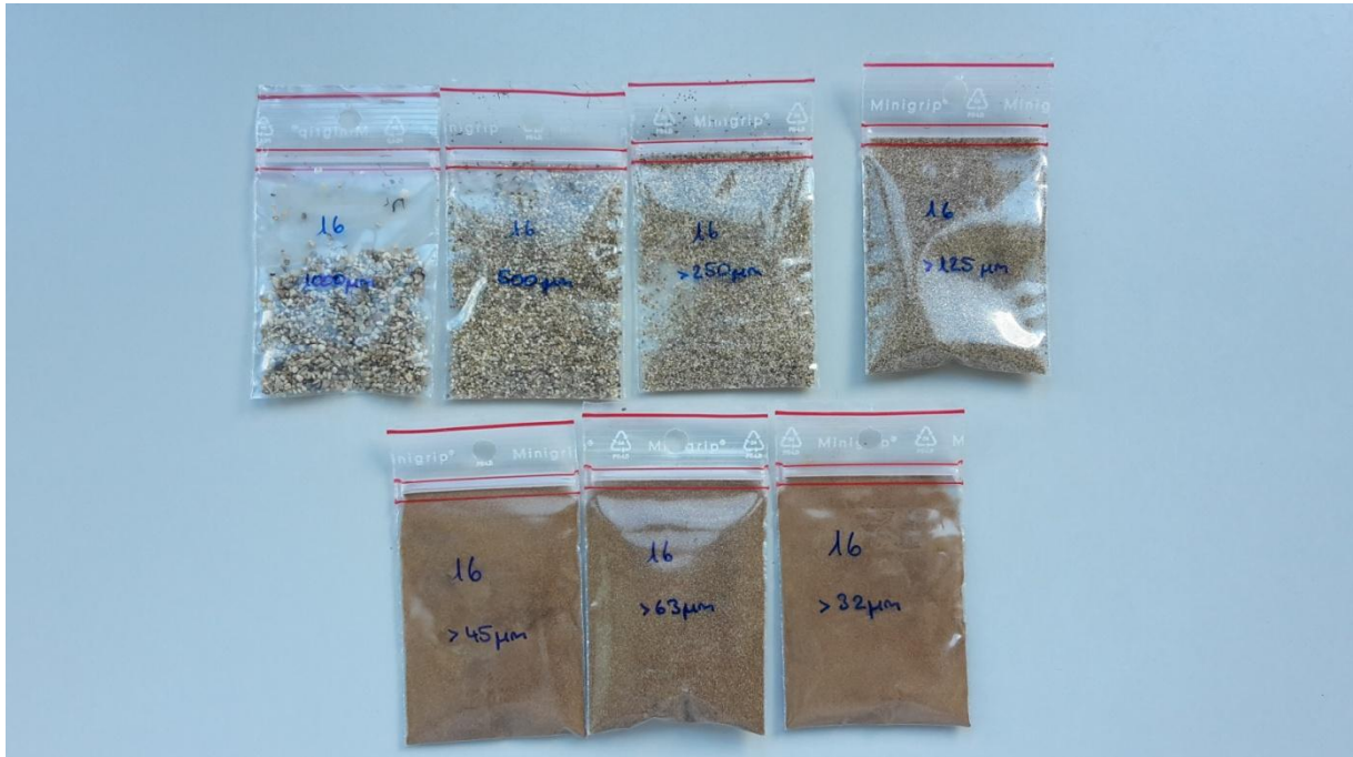
Fig. 2–4: One soil sample split into different grain size fractions. (A. Musso)
