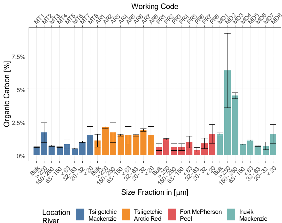
Figure 4-7 Organic carbon ( C_{org} ) in the samples. Colors indicate different measurement sites. The Working code is a unique code identifying each sample. MT refers to Tsiigehtchic / Mackenzie, AR to Tsiigehtchic / Arctic Red, PR to Fort McPherson / Peel and MD to Inuvik / Mackenzie, the number refers to the particle size, with 1 being associated with bulk and 8 with < 20 \mu\text{m} (more details in Table 3-1).
