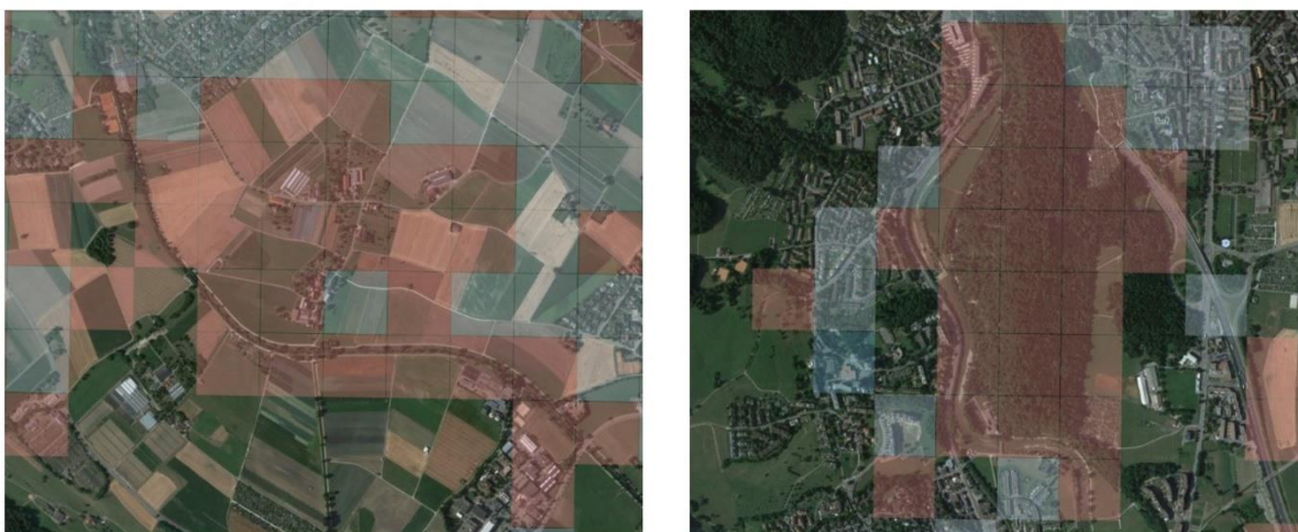
Figure 34 - Detailed examples of disagreements Satellite images with an overlay (transparency = 30%) indicating agreement (blue) or disagreement (red) between the user generated data and the CORINE land cover dataset. The left image corresponds to the highlighted circle number one in Figure 33; The right image corresponds to the highlighted circle number two in Figure 33.
