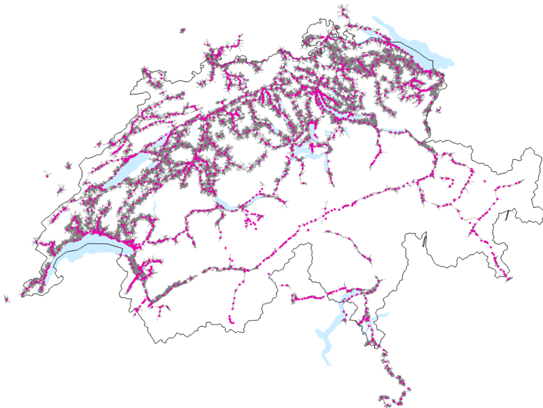
Figure 27 Resulting drive time areas (grey) of train stations (purple) served by the SBB. Drive time areas have been calculated in the direction away from train stations for a 5-minute drive.
