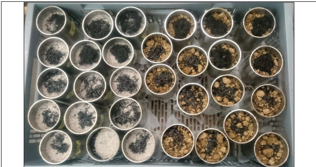
**Figure 7: Field sample preparation.** The charcoal samples were inserted 2cm below the top of the cylinders. On the left are the samples with a sand matrix; on the right the samples with a soil matrix.
