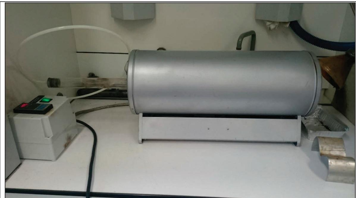
**Figure 4: Pyrolysis oven**, with the quartz glass tube partially inserted. On the left is the hose that supplies the samples with N<sub>2</sub>.
