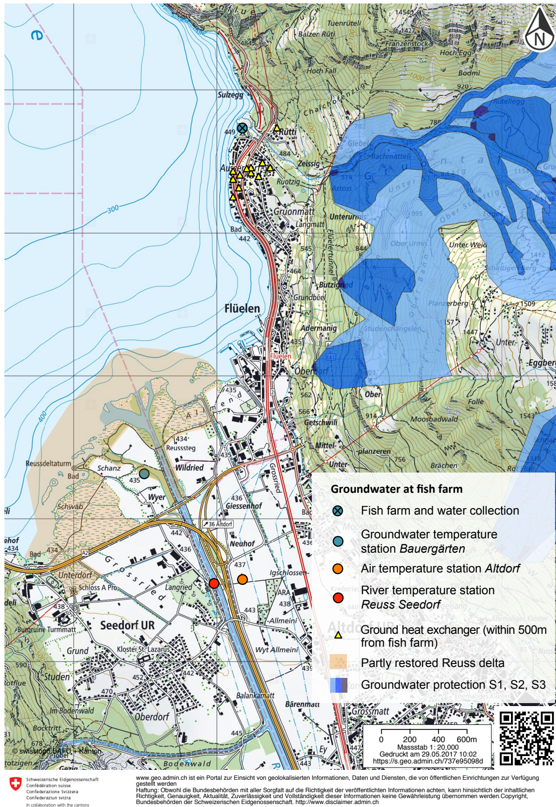
Fig. 13: Fish farm case site, measurement stations and significant influences.
