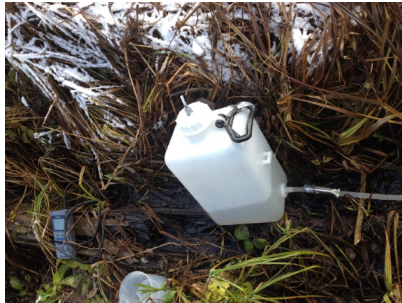
Figure 7: Schematic drawing of mariotte bottle (left: after the new Zealand digital library) equipped with an airtight cap. The only way for air to get into the bottle has to be through the inlet tube. By moving the tube up or down, “H” is in- or decreased and the deliver rate is in- or decreased. The smaller “H”, the smaller the amount of solution flowing out of the bottle. Picture of mariotte bottle in use in Alptal (right).
