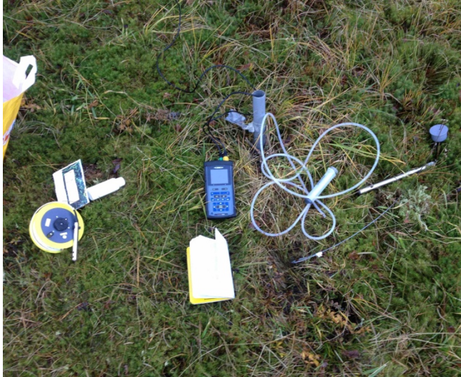
Picture 5: field equipment for ground- and streamwater measurements (left) and for salt tracer measurements (right).
