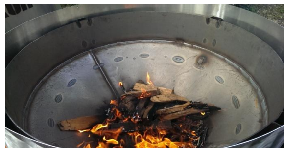
Figure 6: A way to produce biochar with a steel kon-tiki vessel at RiLu Char AG, Schaffhausen (own picture).
