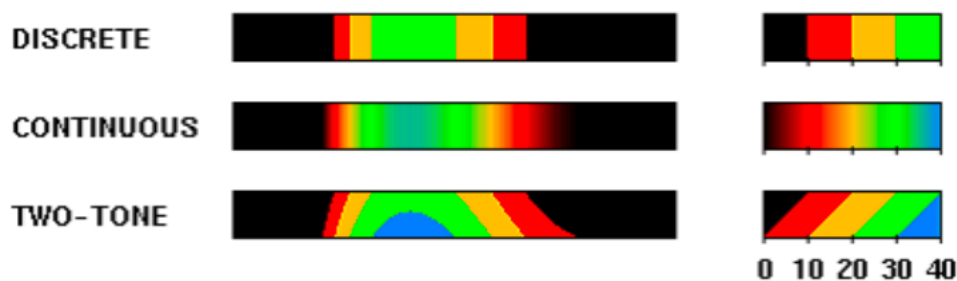
Figure 29: Illustration of a two-tone pseudo coloring scheme in relation to normal discrete or continuous formats (Saito et al., 2005).
