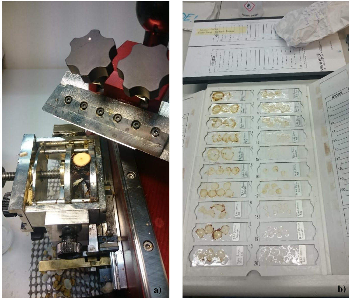
Figure 12: a) Microtome with sample for cross-sectioning; b) cross-sections on glass slides.
