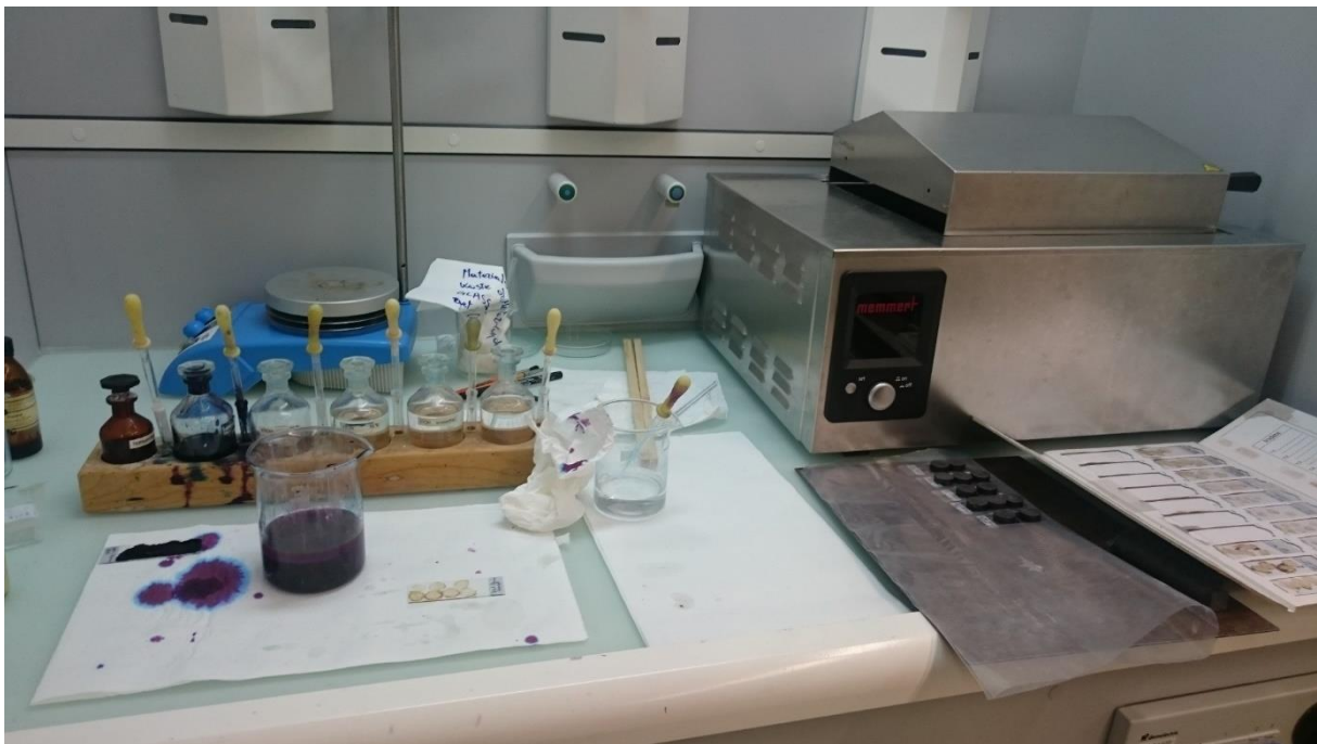
Figure 14: All liquids needed for dyeing; water, double staining solution Safranin and Astrablue, ethanol 75%, 96% and 100% and Xylol.
