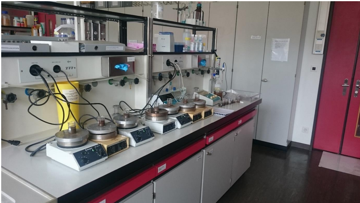
Figure 10: Samples prepared for pH-measurements with a magnet stirrer.
