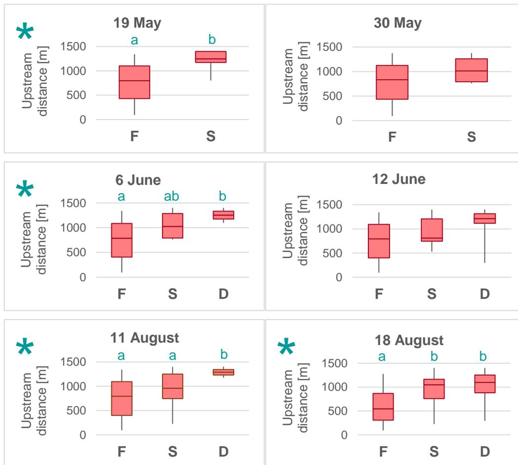
**Figure 33.** Boxplots of the upstream distance for sites with flowing water (F), standing water (S) and a dry channel (D). Statistically significant differences in mean upslope distance for the three different stream states are indicated by a star and different letters.
