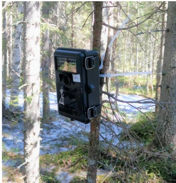
**Figure 8.** Picture of the Bushnell time lapse camera installed in the field (site A3).
