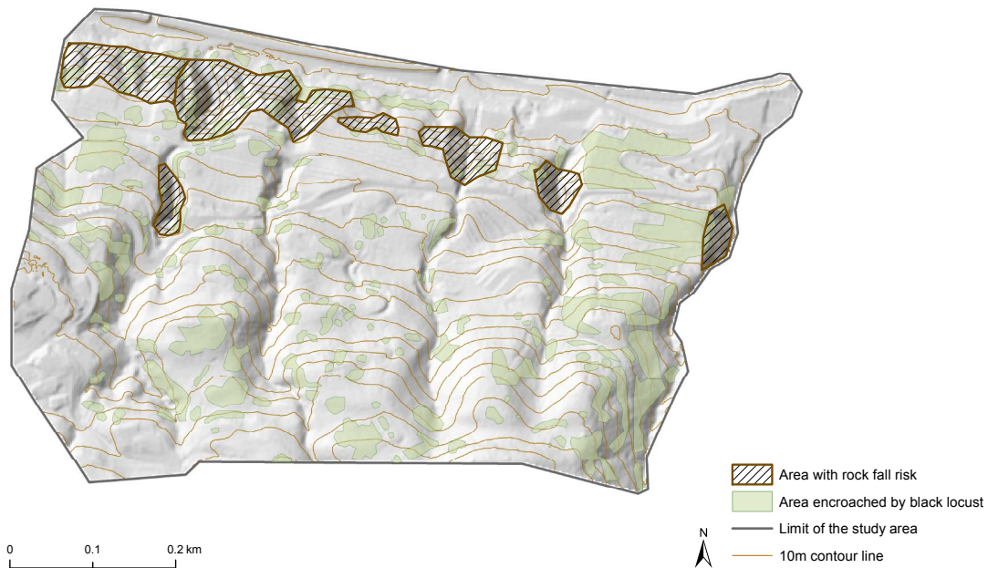
Figure 13: Potential area of the study site of Chiasso affected by rock fall risk
