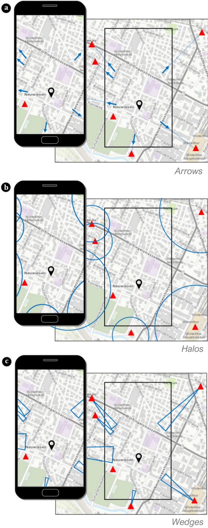
Figure 2: Most commonly used contextual view techniques: a) Arrows, b) Halos, c) Wedges
