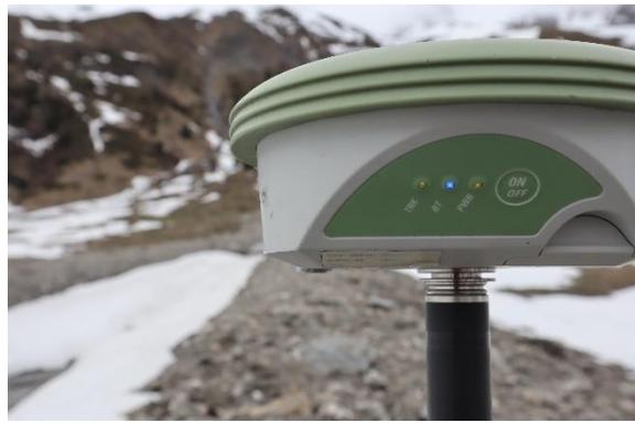
Figure 30: Antenna of Leica GPS1200
