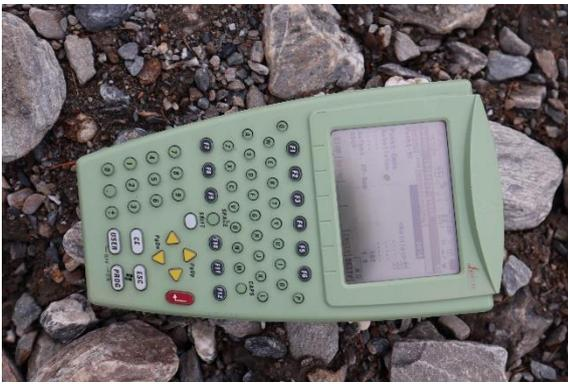
Figure 29: Leica GPS1200
