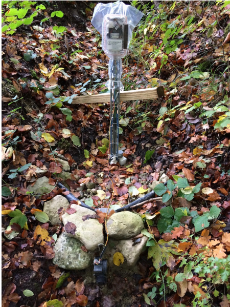
Figure 3.2 Complete experiment setup on an SSS location. The sampler itself is installed on the bottom of the metal rod and covered by a plastic lid which allows for water circulation, while preventing the blockage of the bottle neck by bigger particles carried in the water.
