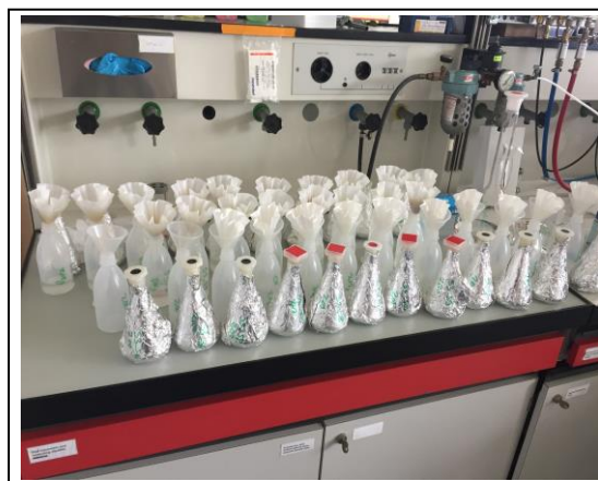
Picture 3: The soil samples shortly before they are filtered and then are already ready for AAS measurement.
