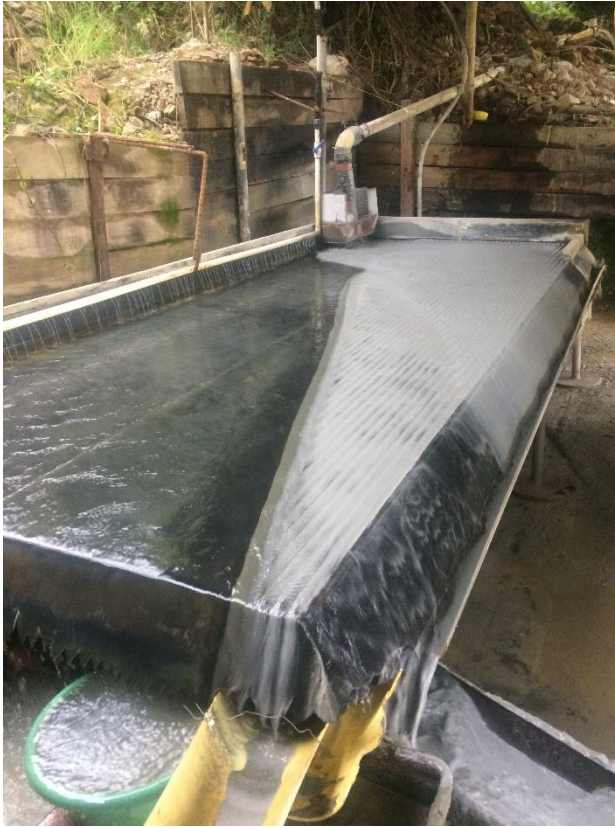
Figure 5: "Shaking table" to separate sand and gold particles through physical process, ASMO 2 (Source: own photo).
