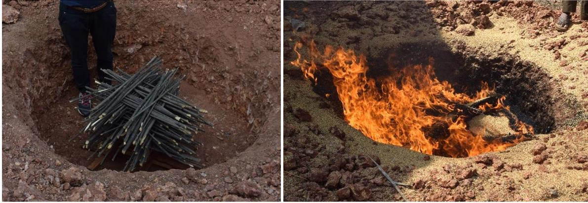
**Figure 6:** Piled up wood to start the fire in the Kon-Tiki (left) and the ongoing production of biochar from rice husk (right) (own pictures).
