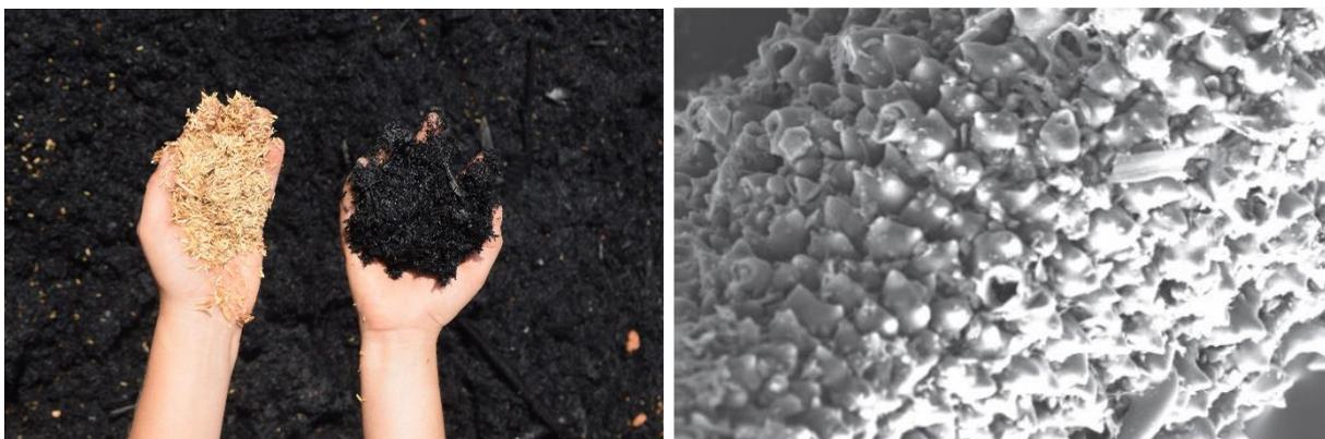
**Figure 2:** Rice husk before and after pyrolysis (left, own picture) and electron microscope image of rice husk biochar with a clearly visible porous structure (right) (Munda et al., 2016).
