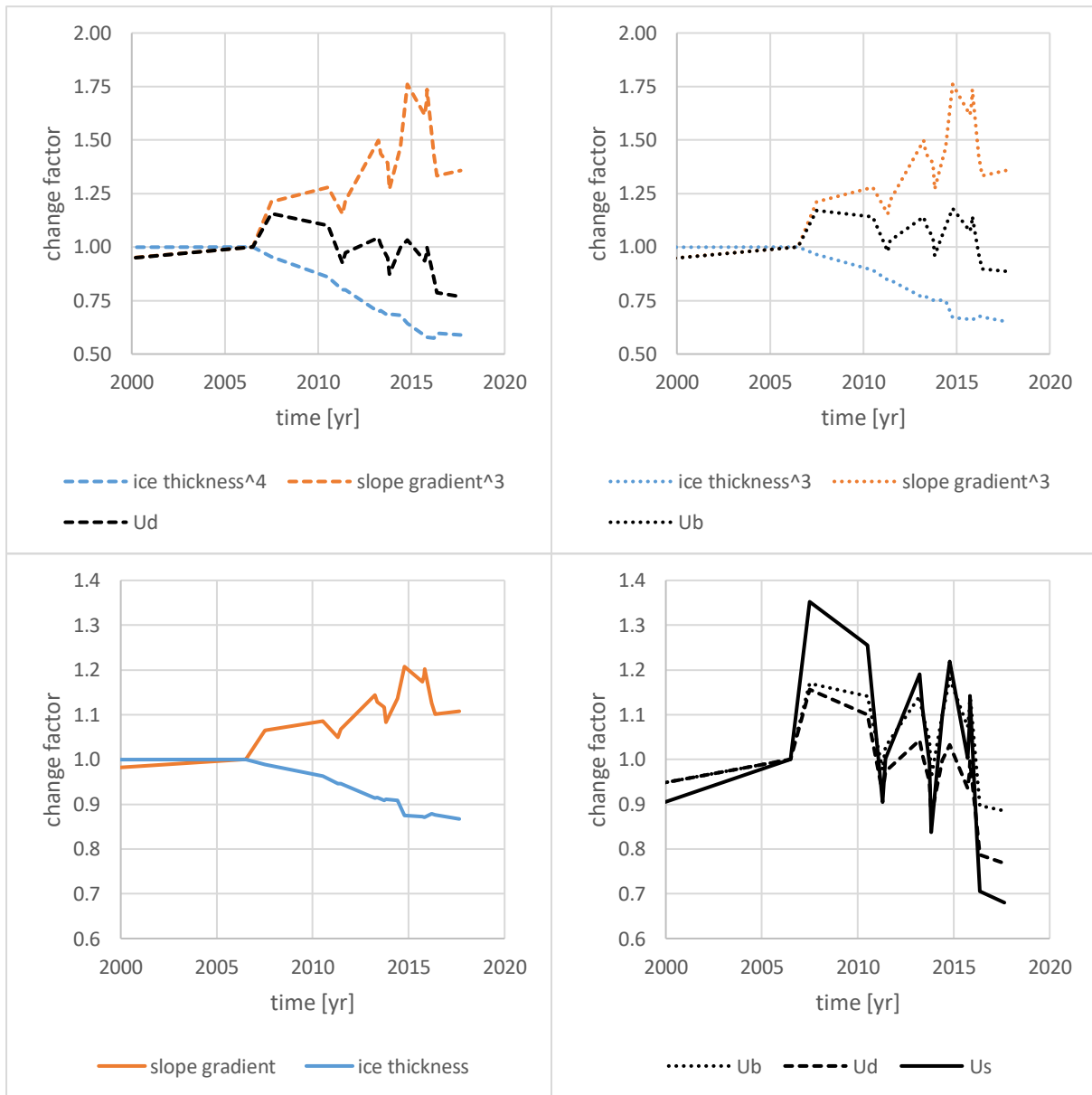
Figure 54: Implications of changes of the surface slope gradient and the ice thickness on the gravitational driving stress (GDS) and accordingly the ice deformation U_d (top left) as well as on the basal shear stress (BSS) and accordingly the basal sliding velocity U_b (top right). The relative changes of the surface geometry lead to a changing slope gradient and ice thickness (bottom left), which results in a (minor) change of the surface flow velocity U_s (bottom right).
