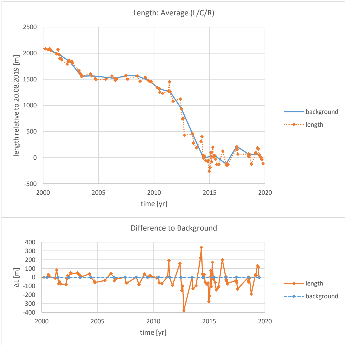
Figure 45: Time series of background length change and seasonal pattern. The values are averaged among the three profiles. A visualisation of the timestamps of the reference fronts for the background change determination is provided in figure 26. Note that the temporal resolution of the front dataset does not allow for a front position seasonality analysis before 2000.
