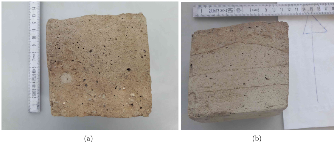
Figure 6: The top of block 1 after abrading the outer layer is seen in (a). The lines scratched into the front side (b) mark where the samples were taken. Orientation is the same as in the field. Note that the lighting conditions influence the color of the blocks in the pictures.
