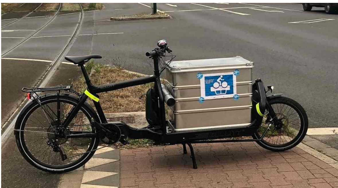
Figure 14: E-cargo bike which does not fit on a pedestrian refuge (Source: Lieb, 2019).
