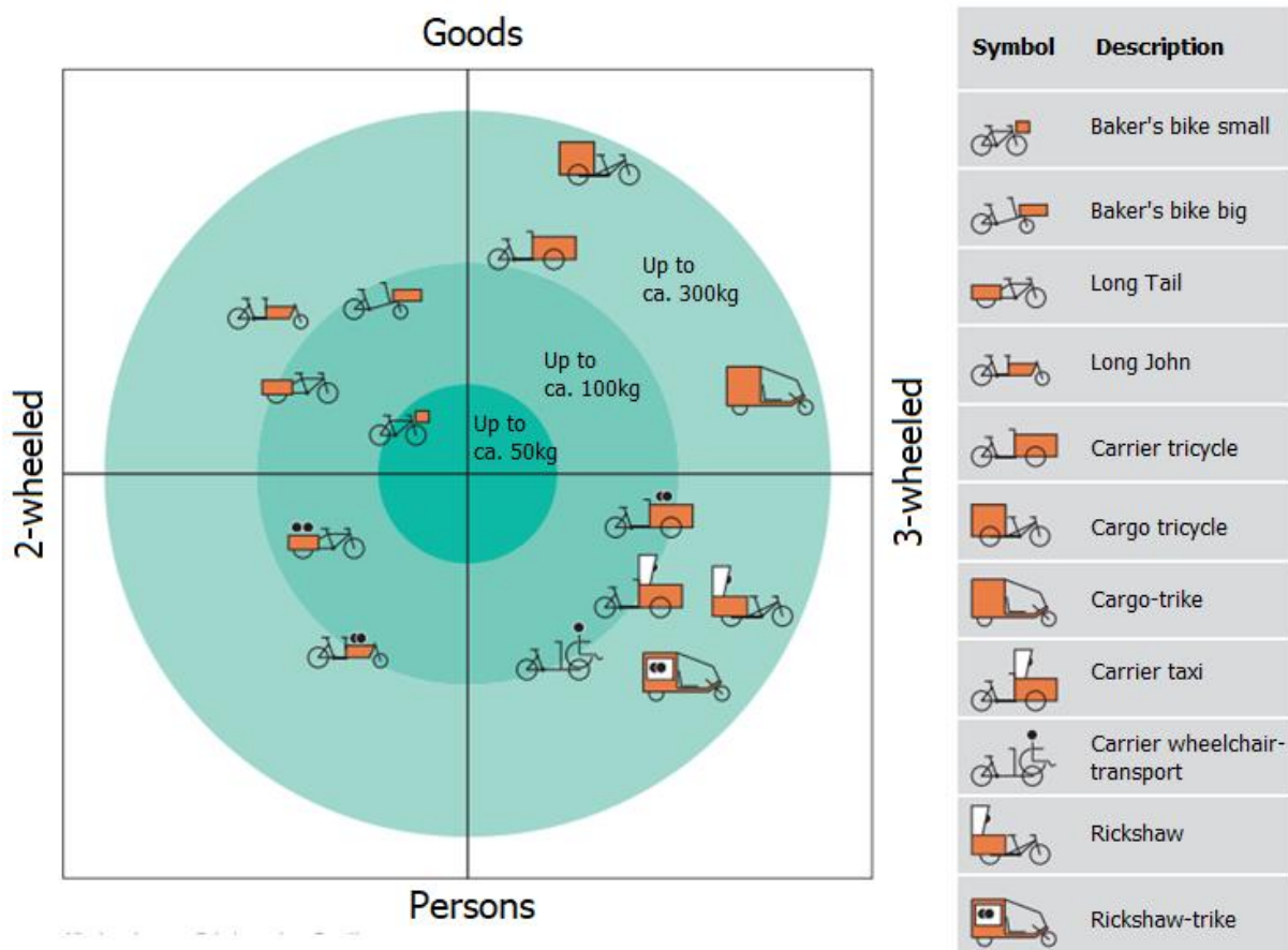
Figure 8: Overview of the different types of cargo bikes (Modified from source: Beckmann et al., 2016, p. 10-11).
