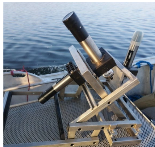
Figure 12: Setup of RAMSES TriOS with the three sensor L_u , L_{sky} and E_d (from left to right) (Picture by Alicia Hug)
