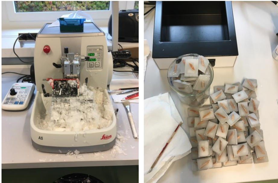
Figure 7: The rotary microtome during the pre-cutting phase (left) and pre-cut samples embedded in paraffin (right).
