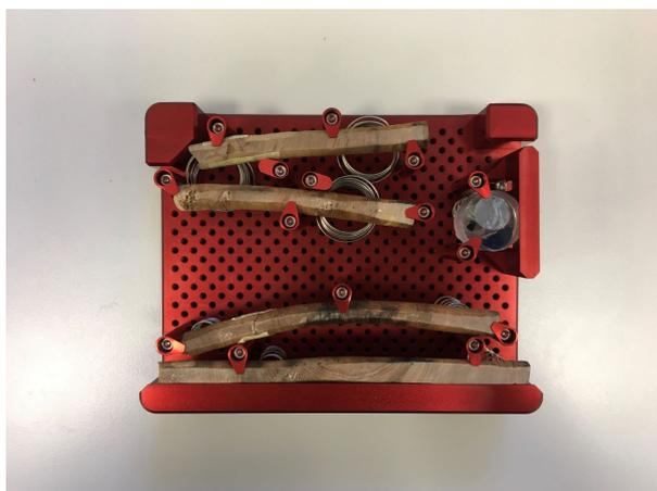
**Figure 18:** The fixed four tree core samples IH01, IH03, IH04 and IH05 together with a standard reference material on the measuring plate viewed from above.
