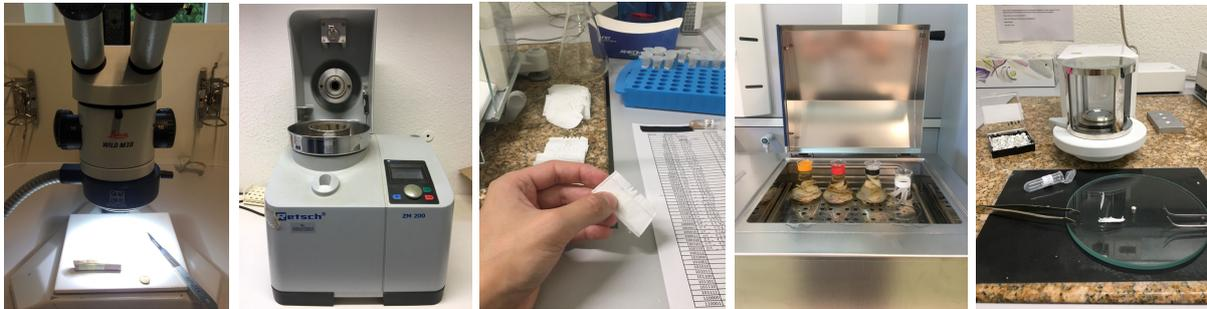
**Figure 20:** The different preparation steps for the isotope analysis (from left to right): splitting the tree cores in blocks of five years with a scalpel under the microscope, milling the block material with the centrifugal mill, packing of the powdered wood material in Teflon bags, the cellulose extraction process in the warm water bath and the final packing of the extracted cellulose material in silver capsules.
