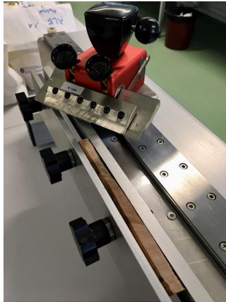
**Figure 16:** Core-microtome with the sample IH05 fixed in the sample holder under the overlying knife holder (red).
