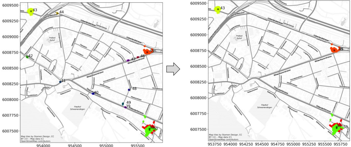
Figure 15 Cleaning of the stop episodes based on minimum time. In this sample image we can see that most of the traffic related small stops are filtered out, as they are not considered meaningful.
