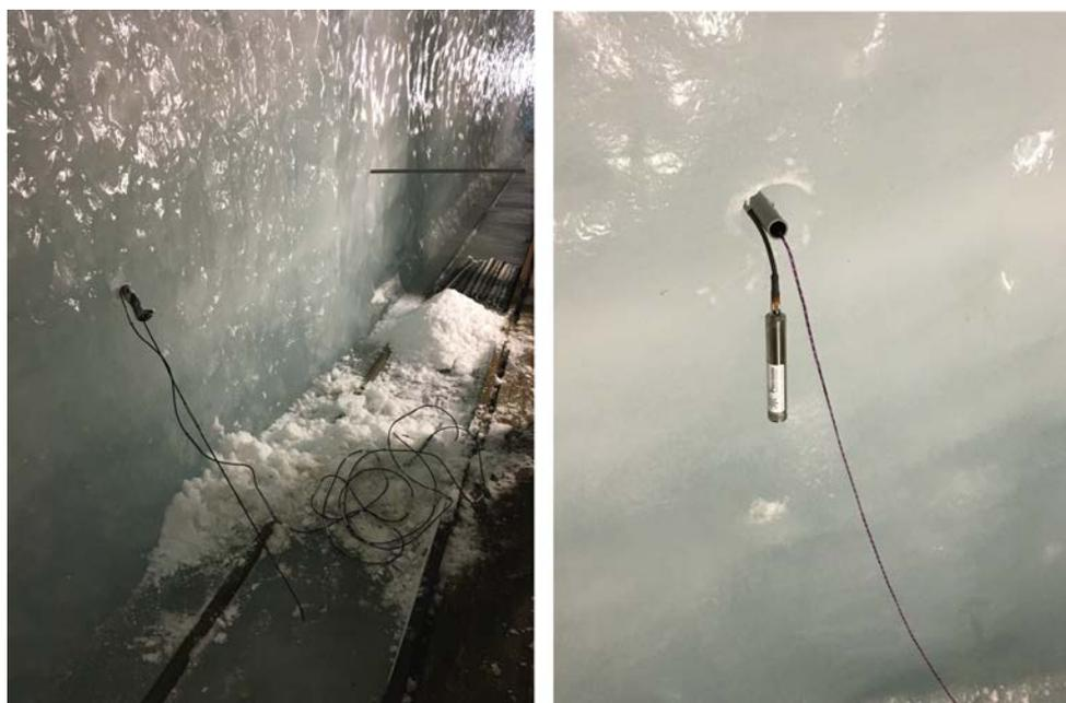
Figure 4.3 – Ice temperature measurements in the wall and in the bottom of the main ice gallery (photo taken on 06.02.2020 (S. Morard)).
