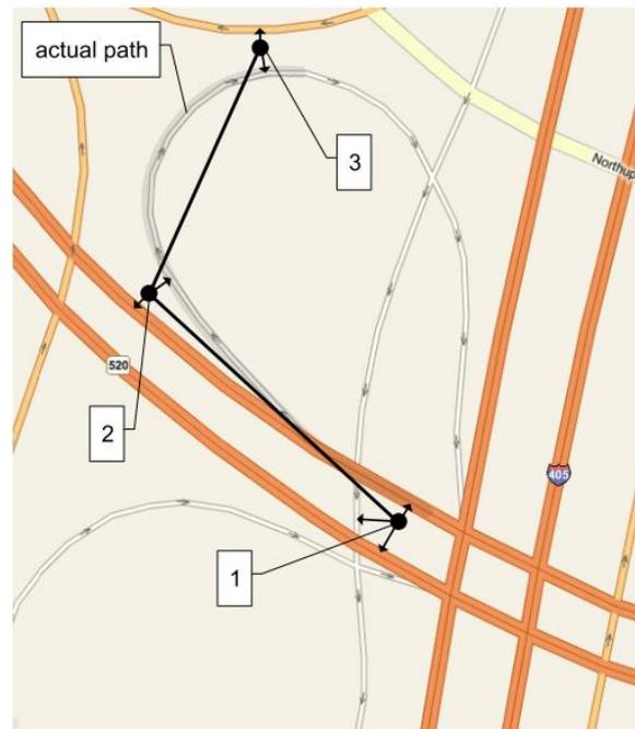
Figure 5: Visualisation of the map-matching problem by Newson & Krumm (2009). The black dots represent the GPS signals and the light grey curve shows the vehicle's actual path. Each dot could be assigned to more than one road segment.
