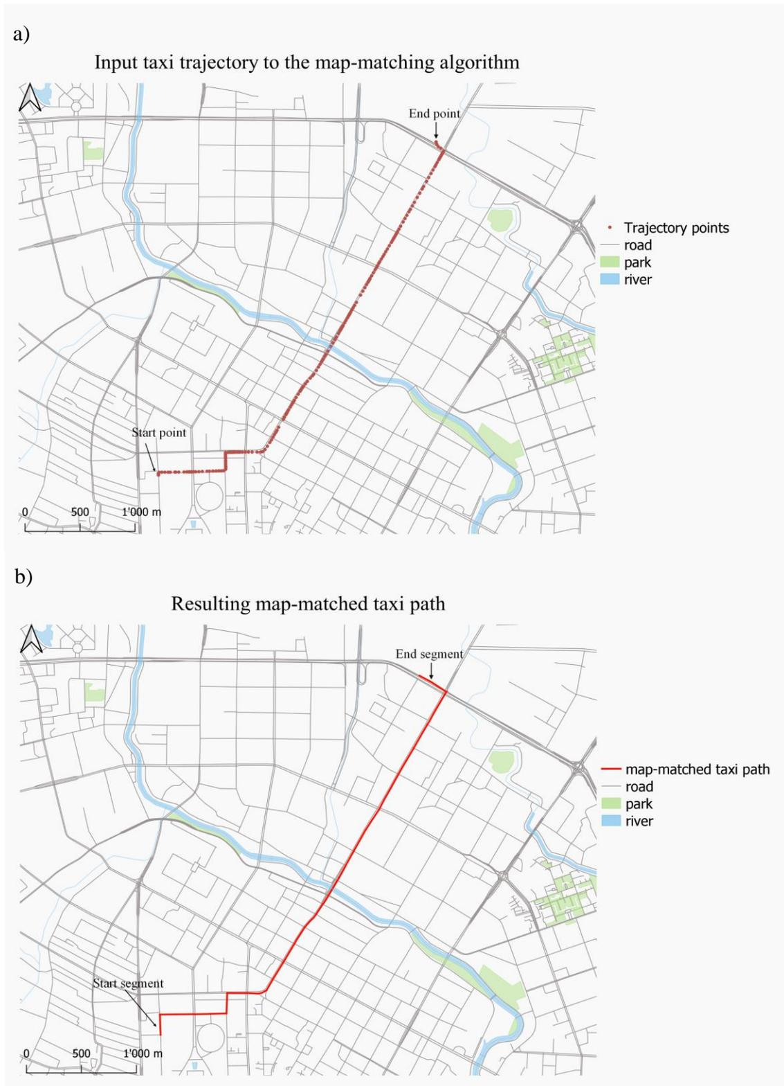
Figure 38: Visualisation of the map-matching result of an example taxi trip. In a) the 320 GPS signals, that are used as the input for the algorithm, are located on the road network of Chengdu. The resulting map-matched taxi path is displayed in b). The start segment of the trip is located south-west and the end segment north-east. The trip consists in total of 42 road segments and is approx. 5.2 km long.
