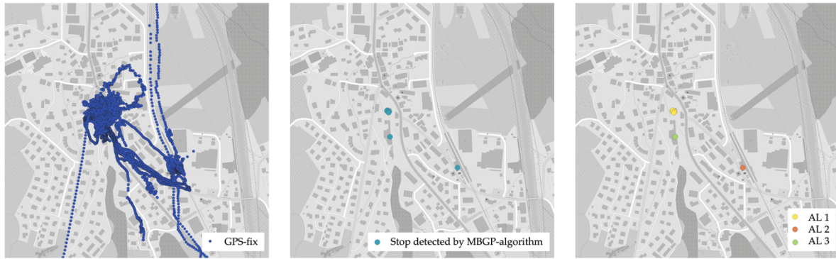
Figure 7: Example of the different steps in AL detection from raw GPS-fixes to Activity Locations (map data from OpenStreetMap)
