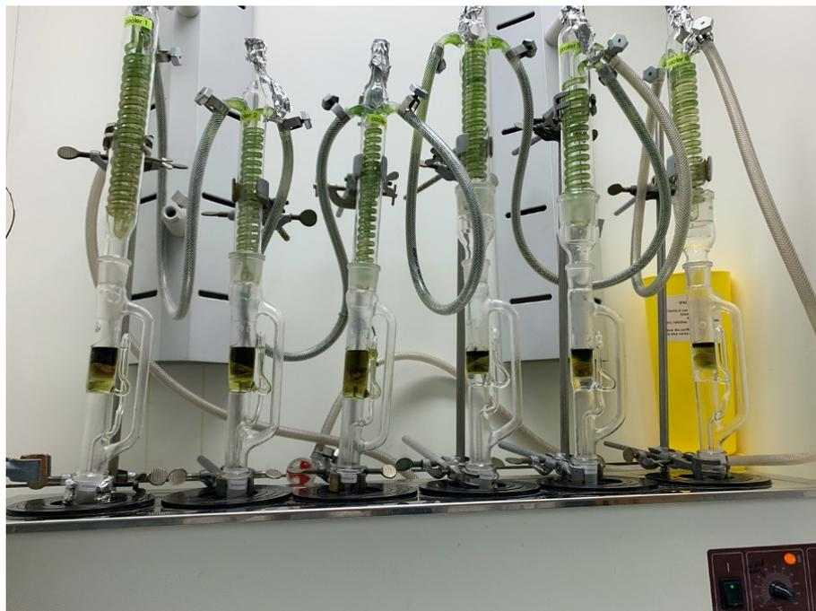
**Figure 5:** Soxhlet extraction apparatus used at the physical Geography laboratory (photograph taken by author)
