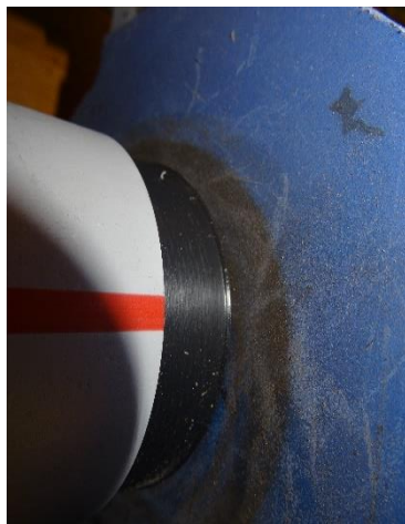
Figure 32: When there is a small bead at the edge of the tube (left) and the thread, the two pieces can gently be pressed together until they hold.
