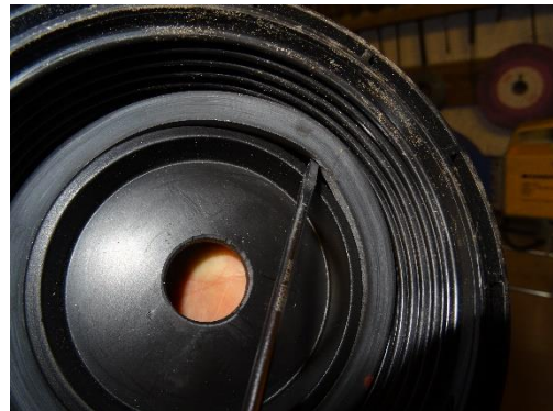
Figure 35: Remove the ring seal with a slotted screwdriver.
