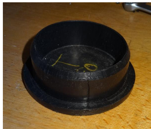
Figure 39: The top cap with one notch in the front. It is suggested to cut more than one notch per cap, in case that one block for some reason.
