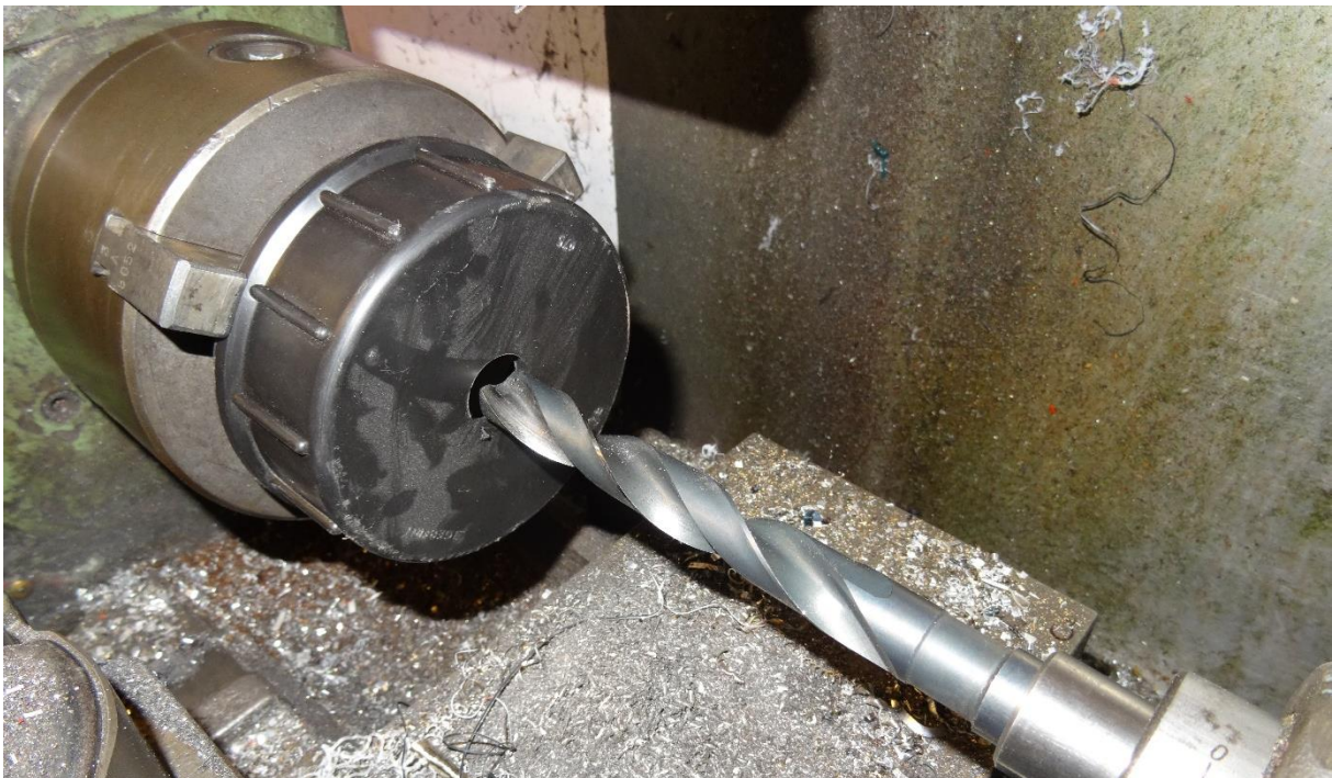
Figure 34: At first, a hole needs to be drilled with a large enough drill bit (depending on the lathe chisel's size), to be able to position the chisel in the hole and enlarge it to the desired width.
