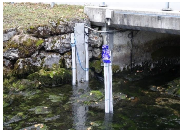
Figure 14: The installation in the Schlichenden Brünnen creek. The reference tube and the tube with the G1/4" thread and O-ring filter are secured to the FOEN monitoring station at the shore, whereas tubes with the G1/2" thread and O-ring and the G1/8" thread and O-ring are mounted to the stake in the middle of the creek. The actual flow was much lower than in the picture provided by the BAFU (Figure 13), but the tubes were installed anyway since the creek was not completely still.
