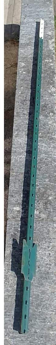
Figure 7: The T-stake with a plate at the lower part, which was used for the field tests.
