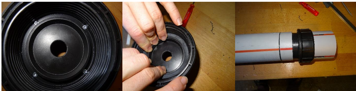
Figure 38: The remaining screws are screwed in (left) before the ring seal is set in place again (middle). The cap can now be screwed on the tube to finalise the tube (right).
