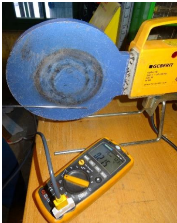
Figure 31: When the temperature of the hot welding plate is between 200 and 220°C the two pieces that need to be welded together, can be held on each side to the plate.
