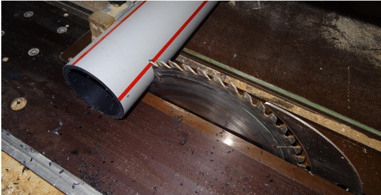
Figure 27: The tube is sawed in three pieces. It is important that the cuts are perpendicular to the tube for the next working steps.
