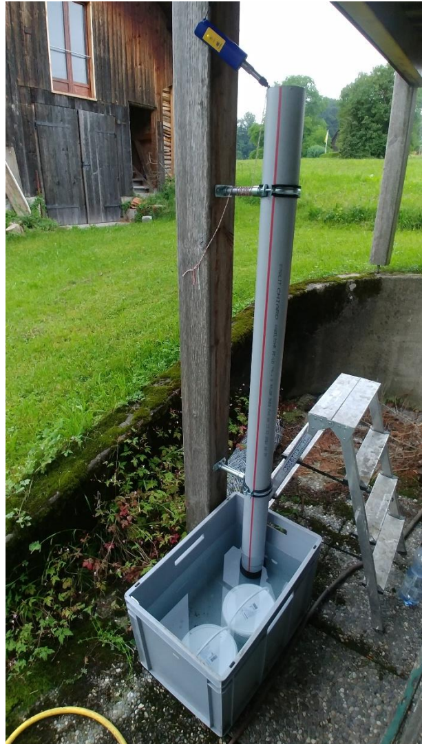
Figure 3: The setup for the first tests. The stilling tube is secured to an immovable pillar over a container filled with water. With the two buckets, the water level was controlled. When these were taken out of the container, the water level decreased by three centimetres.
