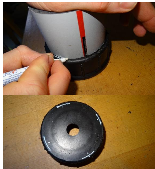
Figure 36: The dimensions of the tube are marked at the outside of the cap (top). Afterwards, the four points are marked 3 mm towards the centre, where the holes for the screws are going to be drilled through (bottom).
