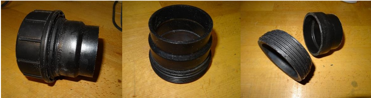
Figure 29: The threaded connector and the cap come in one piece (left). In this step, only the threaded connector (middle) is used. The cut is behind the thread, where the diameter is slightly smaller than at the thread itself.
