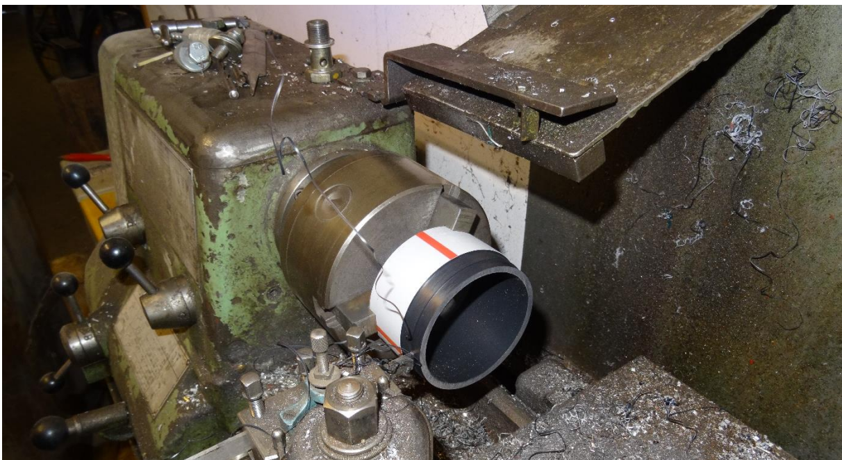
Figure 30: With a lathe, the outer dimensions of the tube can be reduced. Theoretically, it is enough to remove 1 mm of the tube, but to be sure, it is better to remove 2-3 mm, in case the tube is not perfectly round.
