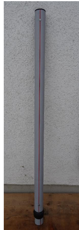
Figure 2: The stilling tube water level recorder. The pressure transducer and desiccant are inside the tube, connected with the cable and the filter is behind the shield at the bottom
