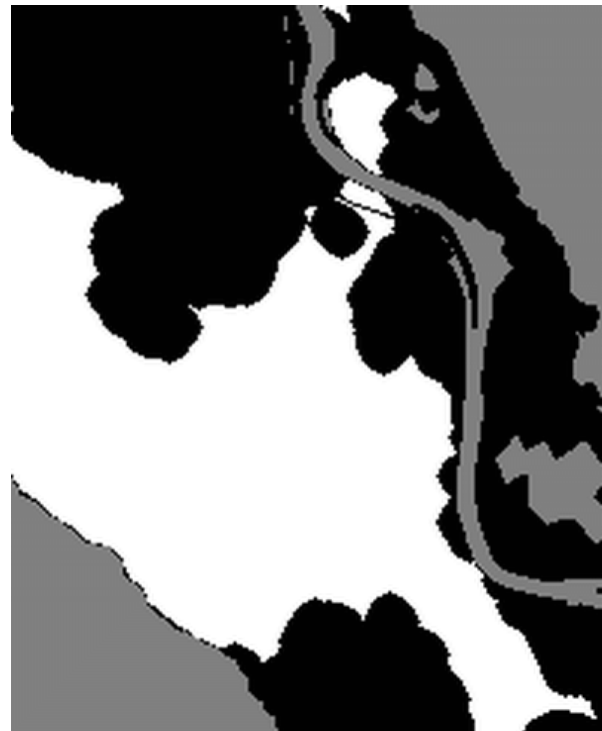
(f) Combined threshold mask after morphological opening
