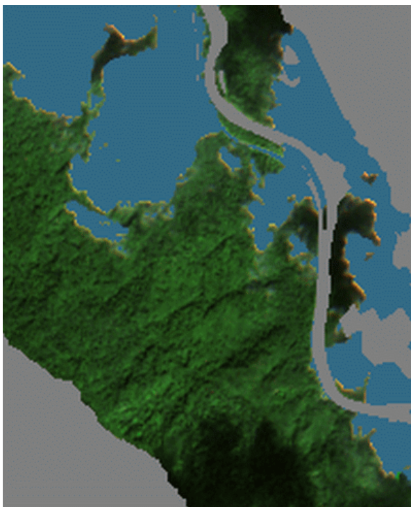
(c) True color composite with threshold applied to the blue band
