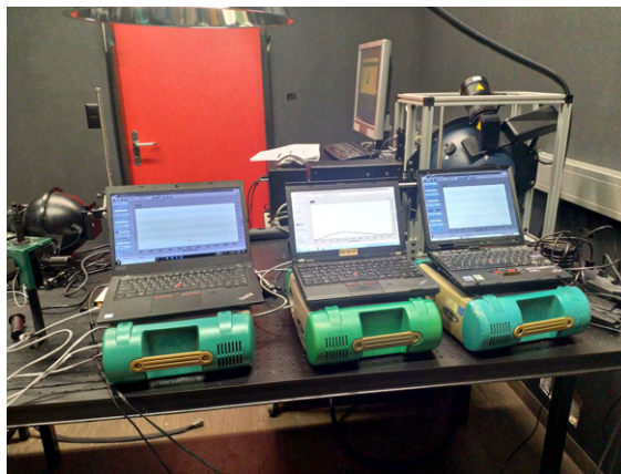
Figure 38: The installation of the three field spectroradiometers for the warm-up experiment and the use of the integrating sphere.
