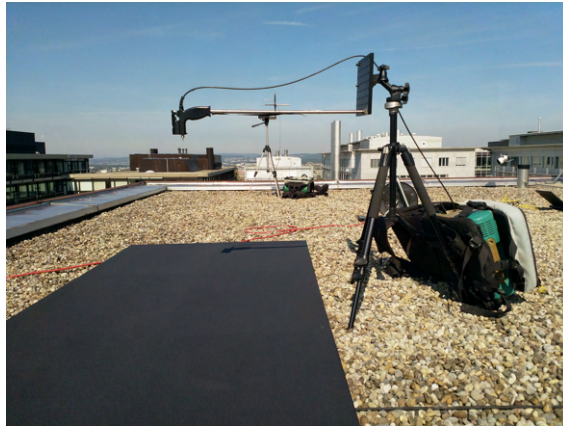
Figure 37: The experimental setup to investigate the matter of the ideal number of target measurements to be obtained.
