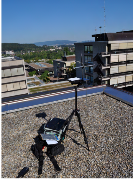
Figure 3: The reference setup installed to collect spectral data.
