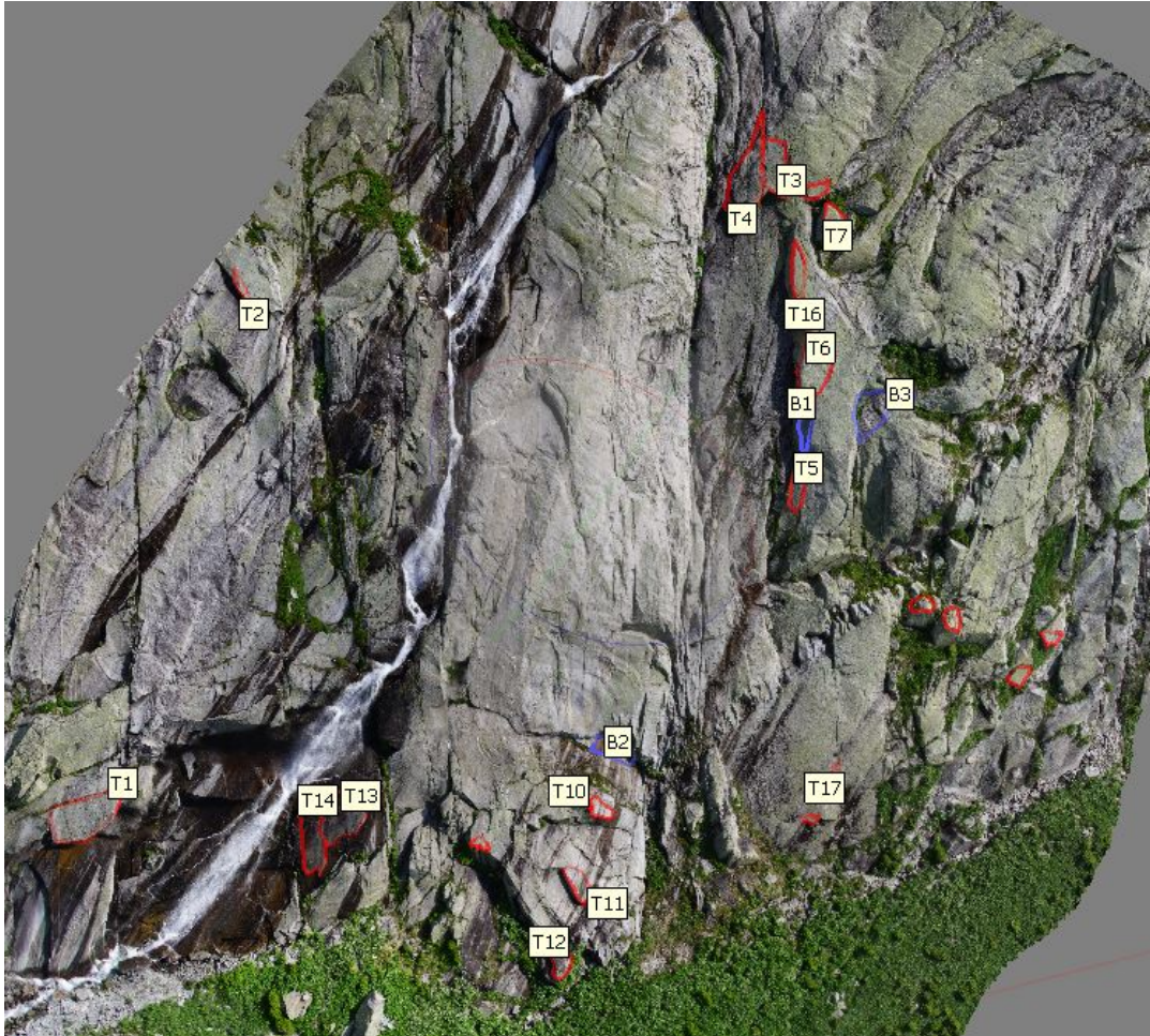
FIGURE 5.17: Existing blocks in the area Lake East. One can observe 19 map blocks in red and 3 missing in violet.
