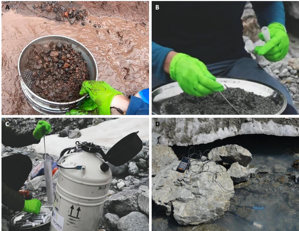
Photos 2 Sediment sampling and measurement of physicochemical stream variables. The sediments had to be A) sieved, B) transferred into cryovials and C) flash-frozen and transported at -80 °C. D) In the meantime, probes were immersed into the stream to measure temperature and conductivity (Photos: Matteo Tolosano (A and C) , Jamani Caillet (B and C)).
