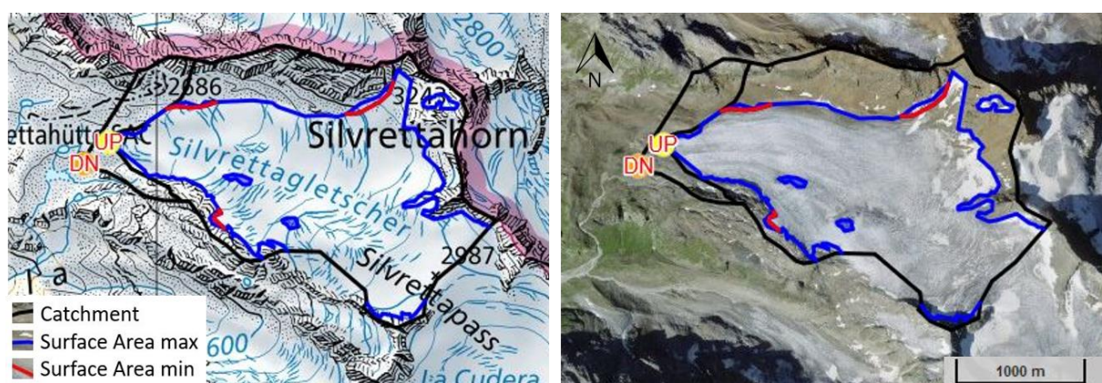
Figure 5 UP- and DN-catchments and maximal vs. minimal glacier surface area polygons at the example of Silvretta Glacier, CH. Map and orthophotos were used as complimentary sources of information about the catchment's current glacierization (modified from swisstopo, 2021a).
