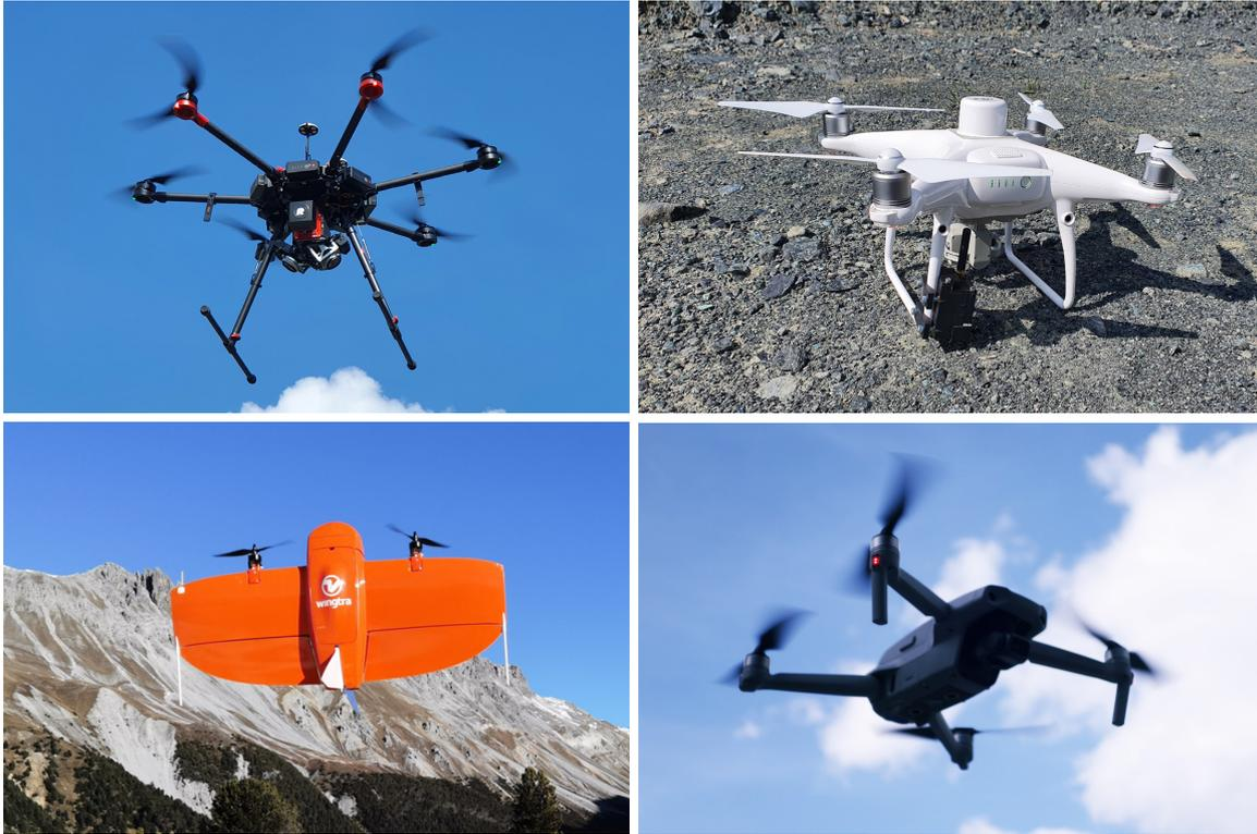
**Figure 4.1.** Different used UAVs: DJI M600 pro with Riegl miniVUX-3UAV, Phantom 4 RTK, Wingtra One, DJI Mavic Air 2 (from upper left to lower right).
