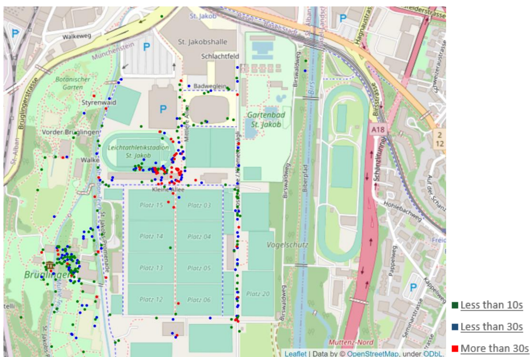
Figure 7: Samsung measurements, stop longer than 5s, less than 10s is green, less than 30s is blue, more than 30s is red
