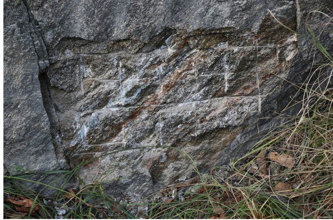
(b) Chessboard pattern on a rock surface cut with an angle grinder before sampling
