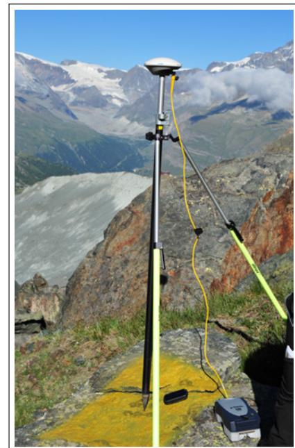
Figure 4.2: dGPS in the field (measuring a ground control point for the Drone)
