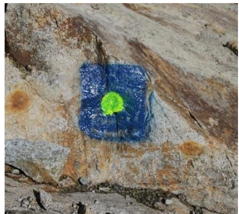
Figure 6: Example of a GCP painted at rocks and stones, which are visible from the time-lapse camera.
