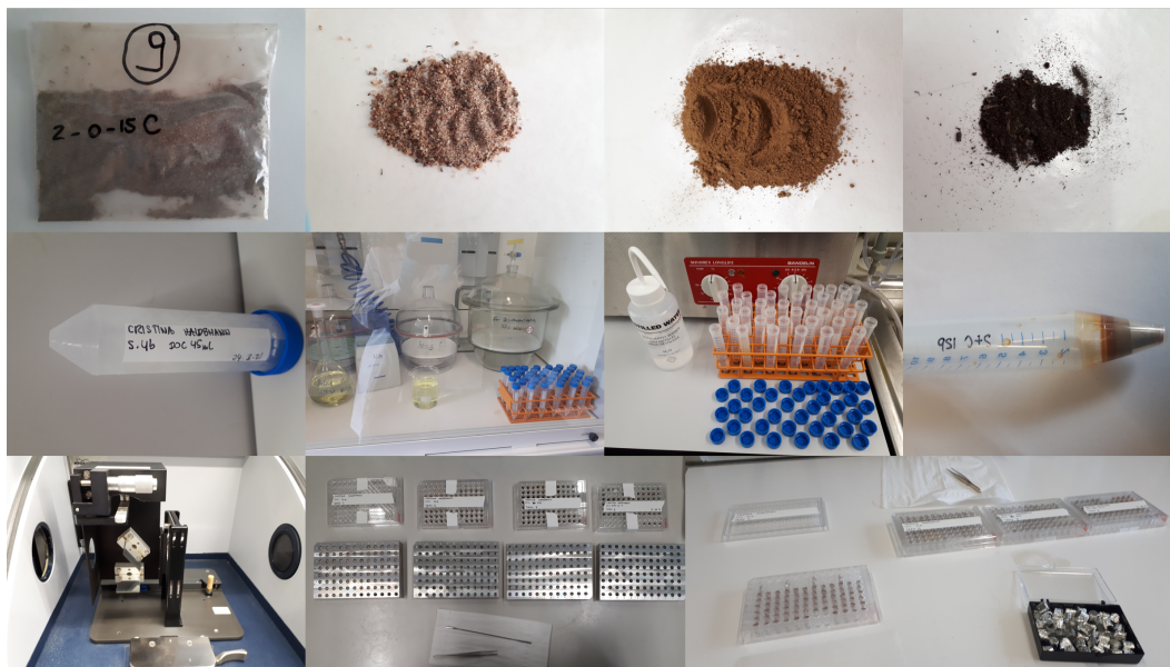
Figure 12: Some impressions from the lab. In the upper line from left: a composite sample, with the consequent sand and aggregate, silt and clay, and particulate organic matter fractions, originated after fractionation. In the second line: the dissolved organic fraction (left) and the extraction of the residual soil organic carbon fraction from the silt and clay fraction. In the lower line from left: DRIFT and chemothermal oxidation at 375 °C.
